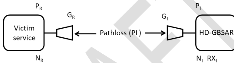
Figure 54: Link budget diagram
